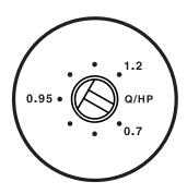
Setting the "Q" is a subtle process. It is recommended that the "Q" setting be left in the 0.7 position and adjusted only after the input sensitivity and highpass crossover ranges are known. Small adjustments to the "Q" setting are all that are required to fine-tune the system.
